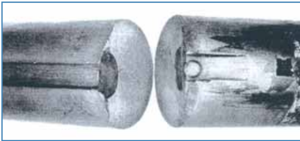
Fig. 1: shaft failure due to fatigue crack (heat treated steel C45)
