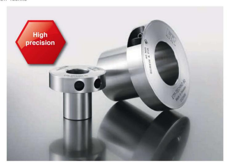
ETP-TECHNO is a hydraulic connection for high precision and frequent mounting. Available as standard for shafts 15 - 130 mm, also imperial. Runout ≤ 0,006 mm.
