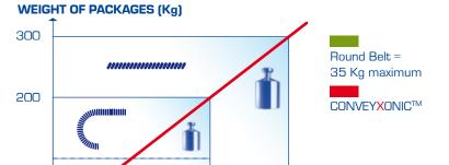
Calculations performed per package weight spread over 4 rollers (rollers of ø 48-50mm)
