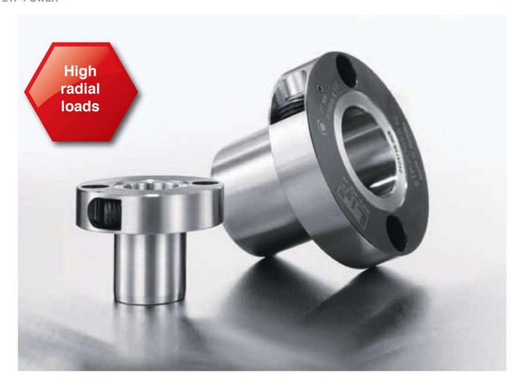
ETP-POWER is available as standard for shafts 15 – 40 mm. Runout ≤ 0,03 mm. Number of mountings 200 - 500 (size dependent). ETP-POWER combines quick mounting with a high radial load capacity due to the specially developed pressure medium.
