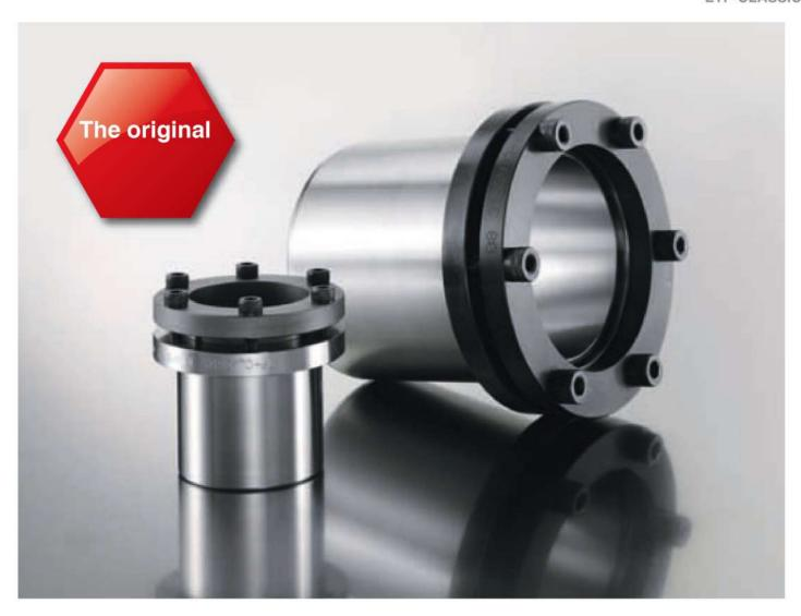
ETP-CLASSIC is available as standard for shafts 15-100 mm, also imperial and a short version, (type S). Also available in stainless steel (type R). Runout: 0,03 – 0,06 mm. Number of mountings: 100 (type R: 50). The small number of clamping screws
